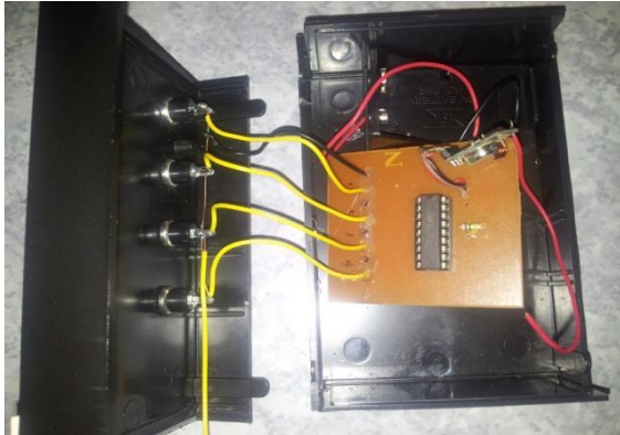
Fig5.1 RF Transmitter Circuit
