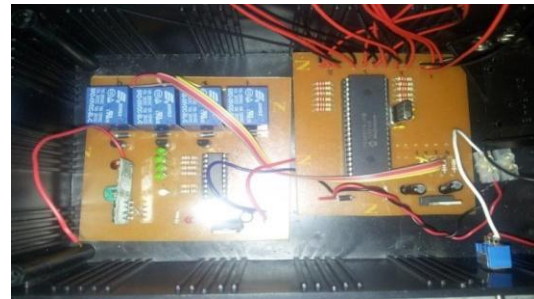
Fig 5.4 Traffic Light Circuit
